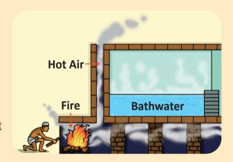
Roman baths had special **tunnels** under the floor. These tunnels were typically made using **brick** and clay. The hot air from the furnace circulated through the tunnels under the entire bath, keeping the floor warm. The heated floor then kept the bathwater nice and warm.
